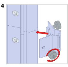
Using the screws provided, attach 8 of the brackets to the joints of your verticals and two at the top of you PMFC2 verticals.
